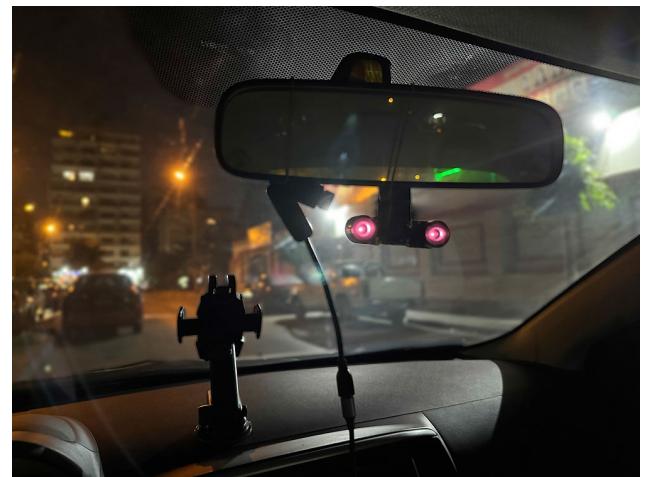
FIGURE 13. Real world testing setup with IR camera mounted in vehicle.
